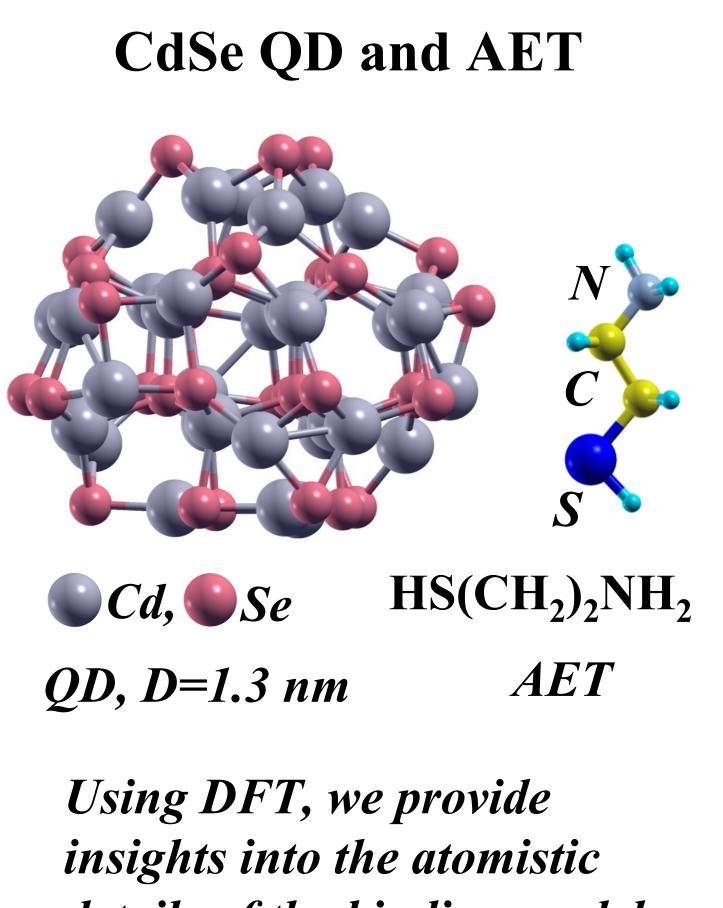
details of the binding models of the AET molecule on the CdSe QD surface.
